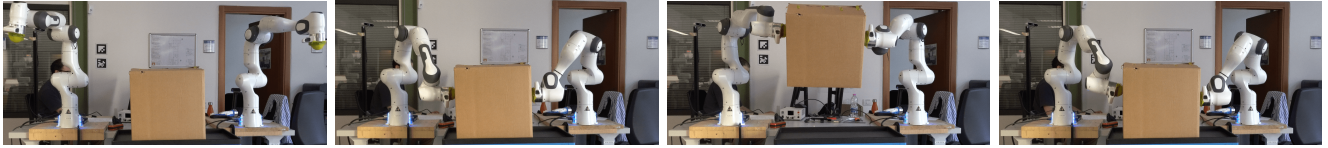
Fig. 7. Snapshot of a pick-up task. The robots start from the initial configuration and reach the estimated contact points provided by the vision layer. Then the framework starts to apply force and lift the box. In the end, the system put down the box in the original position.
